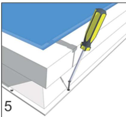
5. INSERT INOX SCREWS, 3.9 X 25MM, USING A CORRESPONDING SCREW BIT. PREFERABLY USE AN ELECTRIC DRILL AT LOW FORCE
