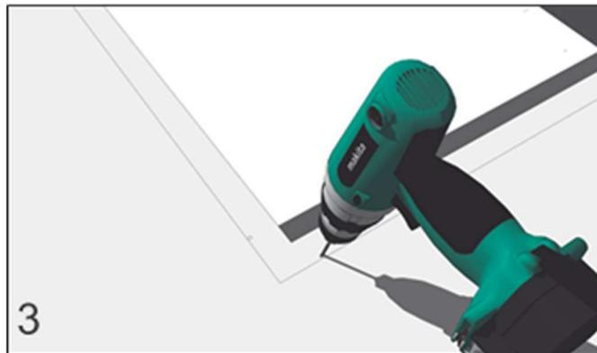
3. DRILL THE MARKED HOLES WITH A 6MM DRILL BIT AND INTRODUCE 6 MM DOWELS.
