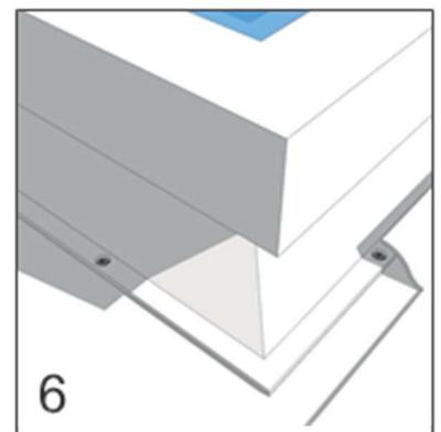
6. PERFORM A WATERPROOFING LAYER ABOVE THE SKYLIGHT BASE. IT IS IMPORTANT TO CARRY OUT THE SEALING, SILICONE CAN DEGRADE OVER YEARS
