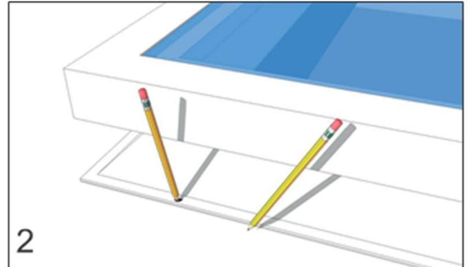
2. MARK THE HOLES IN THE BASE WITH A PENCIL OR FINE DRILL BIT. MARK THE OUTSIDE EDGE OF THE BASE
