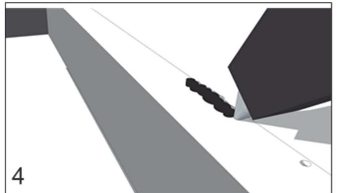
4. APPLY A SILICONE CORD OF APPROX. 1CM ON THE INSIDE OF YOUR MARK. FILL UP BREADS WITH SILICONE, USING POLIURETHANE SILICONE
